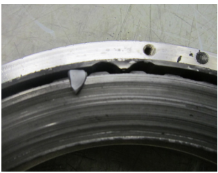
Stationary carbon beyond repair will be reverse-engineered
