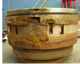
Heavily contaminated dry gas seal from N. American refinery
