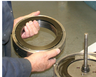
Dry gas seal disassembled for inspection
