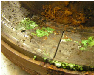
Fractured carbide rotating ring, and decompressed O-ring
