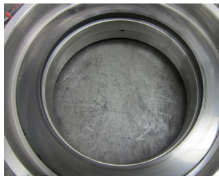
Replacement stationary seal ring ready for re-build and test
