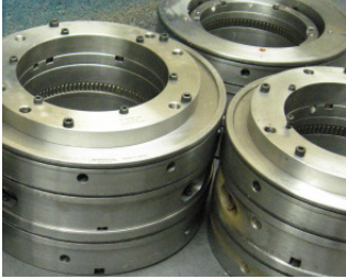
Dry gas seals returned for repair from African methanol plant
